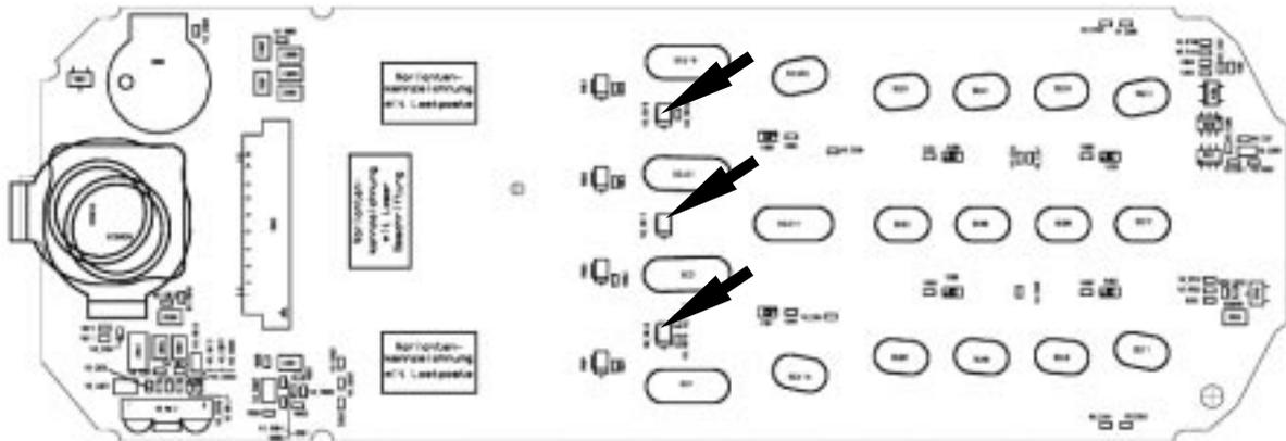
Figure 4: S25 board display LED placement and polarity
