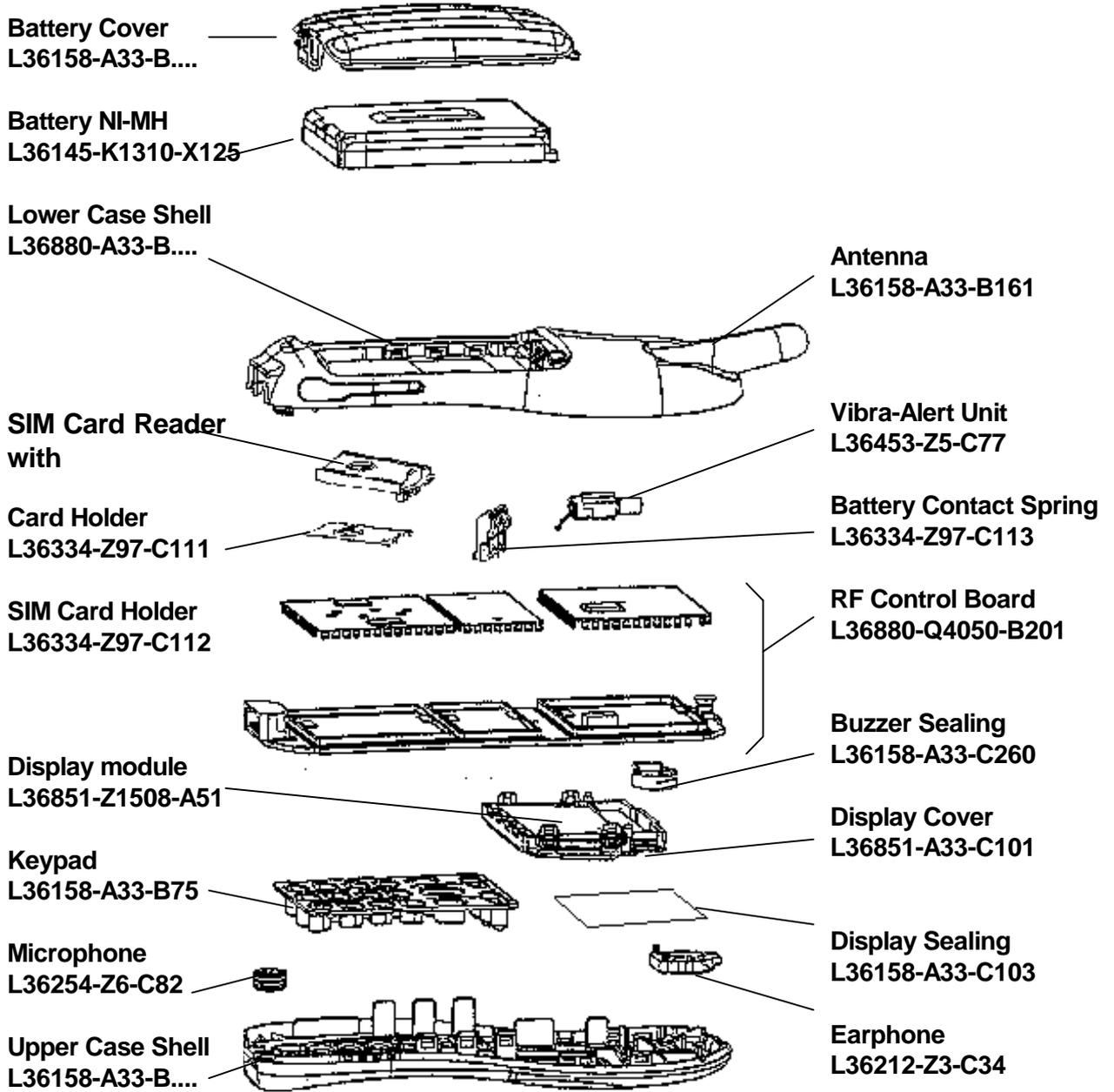
*Disassemble the C35*
