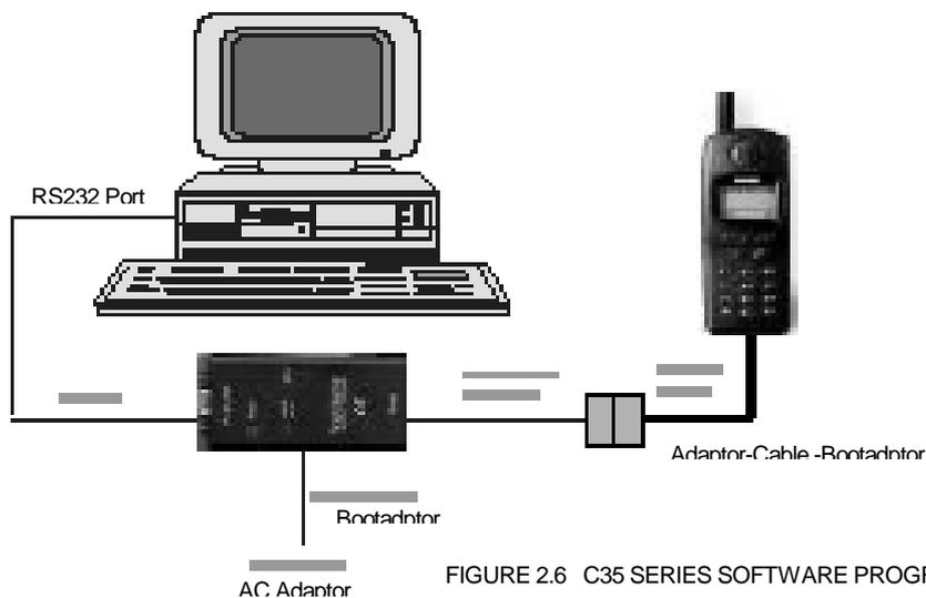
FIGURE 2.6 C35 SERIES SOFTWARE PROGRAMMING SETUP
