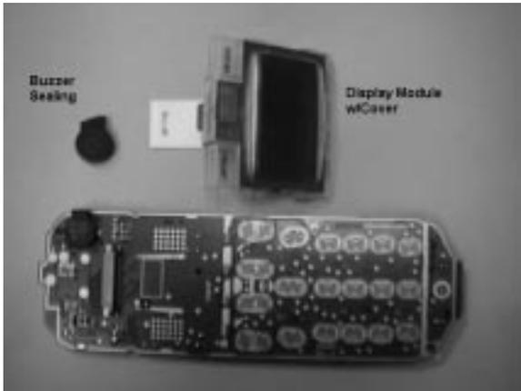
PHOTO 2.11 Disassemble Control Board Assy – STEP 2
