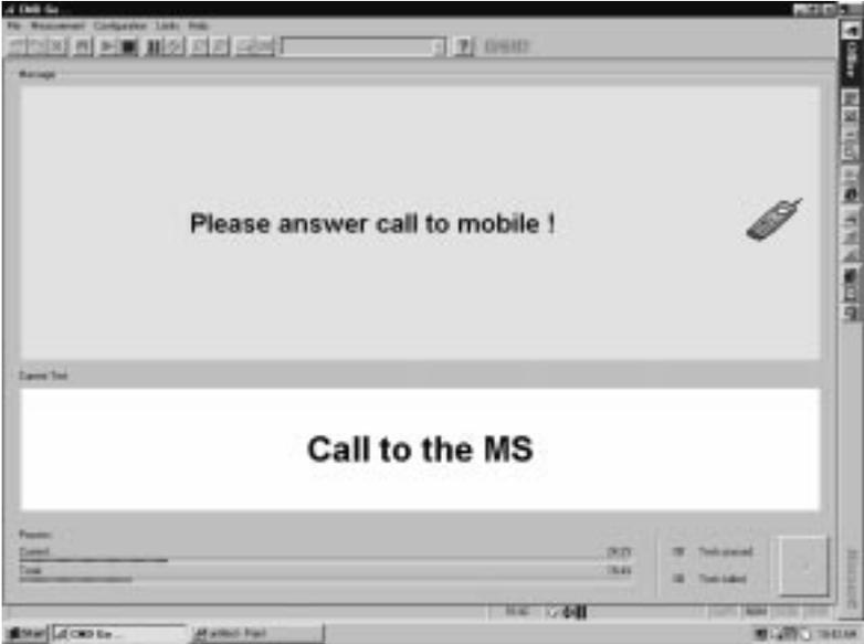
Next, the GSM test set will end the call to the mobile phone and the screen will prompt for Dialing from the mobile phone. At this test step, please move the mobile phone to the Antenna Cradle and switch the RF switch to EXT ANT position. Once the mobile phone log to the GSM test set, dial 1234 and the Send key.
