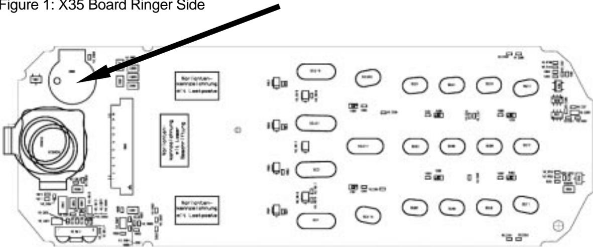
Figure 2: X35 Ringer (B800) Placement (Top View)
