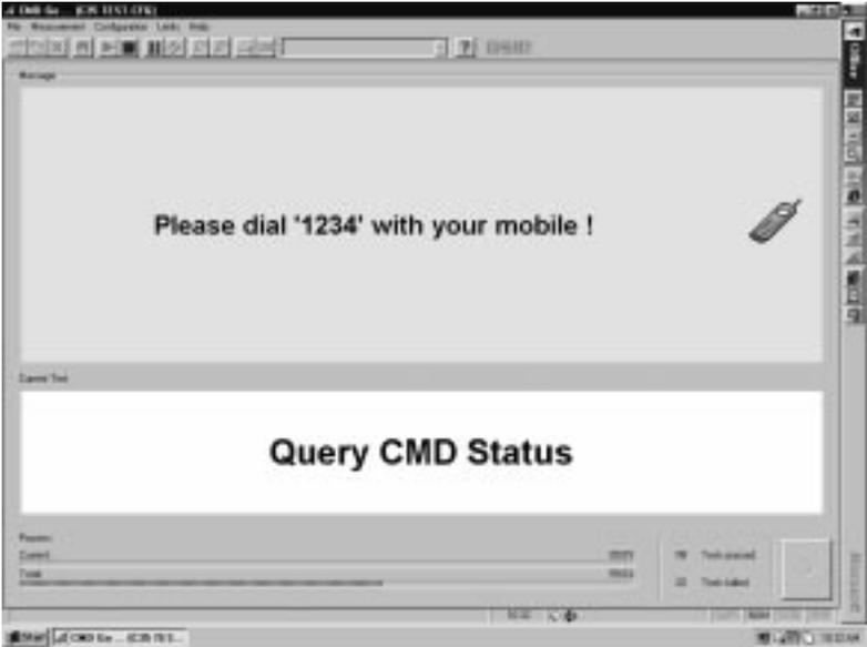
The GSM test set will make Tx Power measurements, Rx BER measurement, Echo Loop test on the GSM and GSM1800 channel specified by the configuration setting. There will be 2 Echo Loop Back test for checking the speech quality – one for GSM and one for GSM1800. Speak into the mobile phone when prompted and listen the voice after appr. 1 second and check the speech quality. If not O.K, it may be microphone or the earphone defective.
