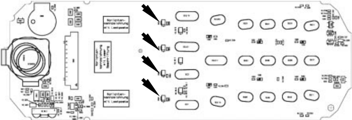
Figure 2: C/M35 board display LED placement and polarity
