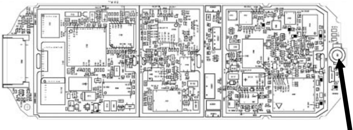
Figure 1: X35 Board Antenna Connector Side (Top View)
