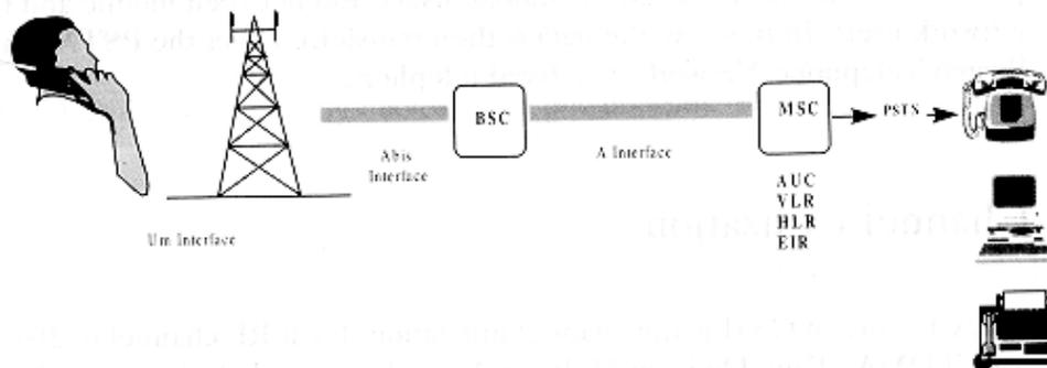
FIGURE 1.2 GSM ARCHITECTURE
